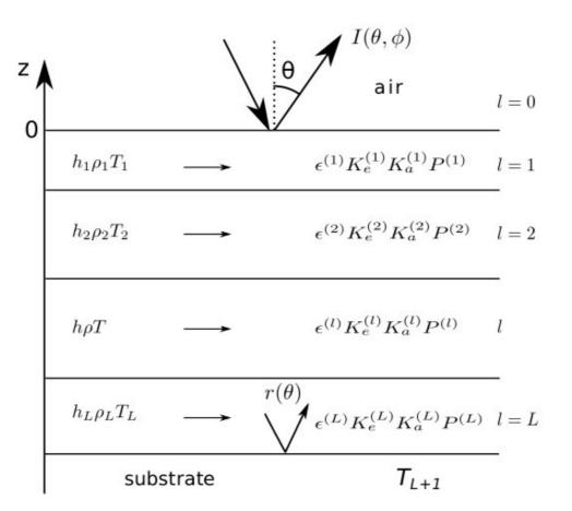
Layers are not necessarly « smooth » from the EM point of view, they can be rough, but for the propagation of energy (RT) perspective, they are parallel
